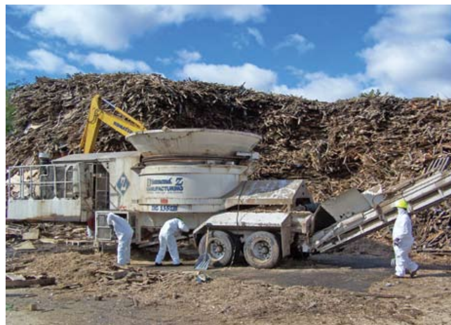
The scrap wood removed from commercial customers is shredded and manufactured into quality colorized mulch sold to landscapers and garden centers.
